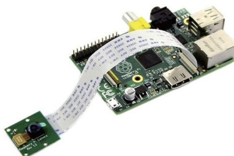
Connection of Camera module on Raspberry Pi board
